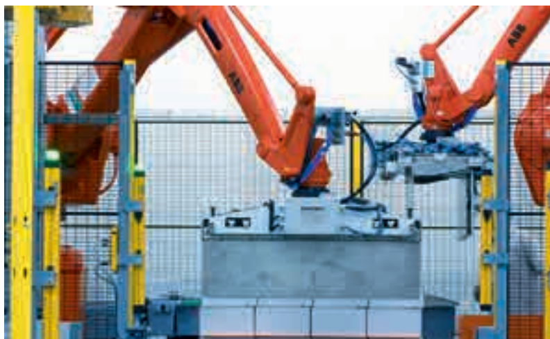
Palletisation unit comprising 2 robots that palletise boxes and shrink packs fully automatically according to 15 different stacking patterns.
